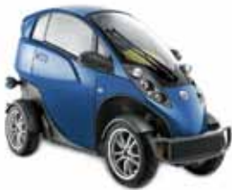
Smera by Lumeneo 98 cm wide, 250 cm long 500 kg 110 km/h, 0-100 km/h in 8 s Driving range 100 km www.lumeneo.fr
