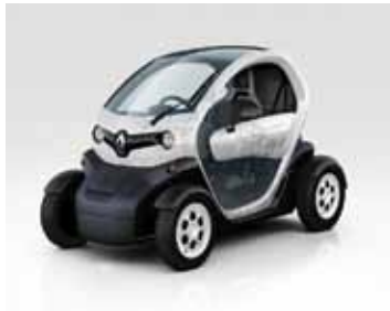
Twizy by Renault 119 cm wide, 233 cm long 450 kg 75 km/h Driving range 100 km www.renault.com
