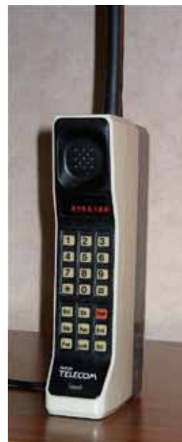
© Wikimedia Mobile phone from the mid-eighties: 35 cm high and 800g for a cost of 4000$.
