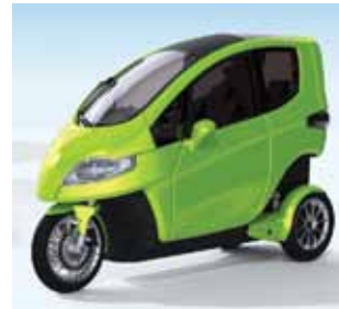
Tilter by SynergEthic 90 cm wide, 253 cm long 340 kg 110 km/h, 0-100km/h in 13 s Driving range 120 km www.tilter.fr
