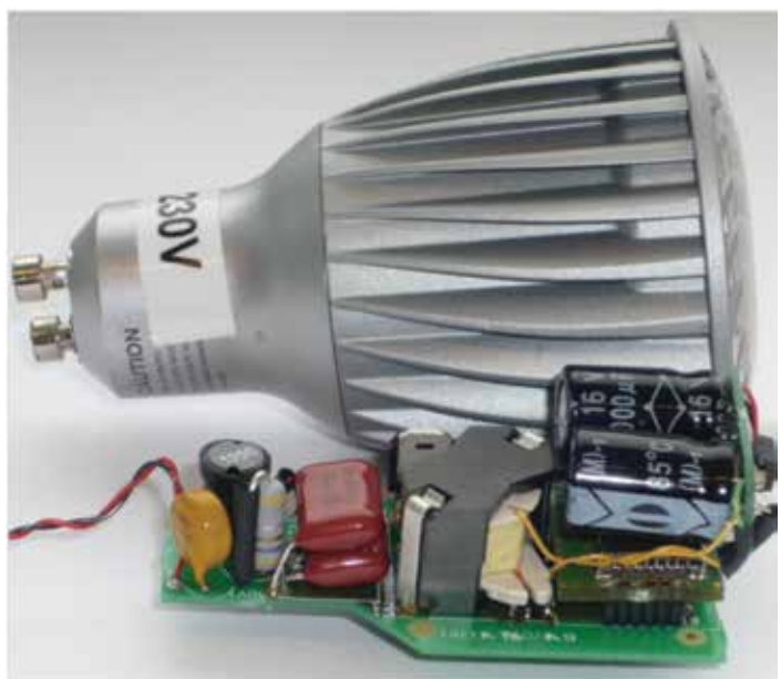
Fig. 4: NXP smart lighting module for 230V GU10 MR16 LED lamp
