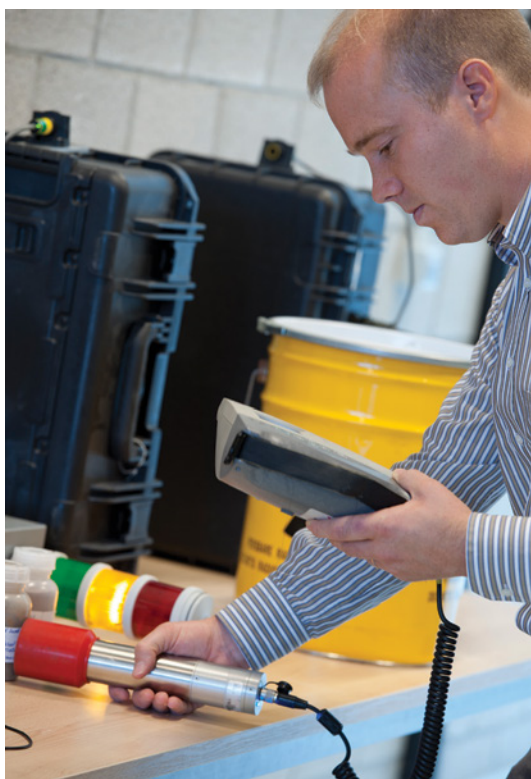
Wouter Schroeiers measuring NORM residues. A small detection portal for radiological material in the background
