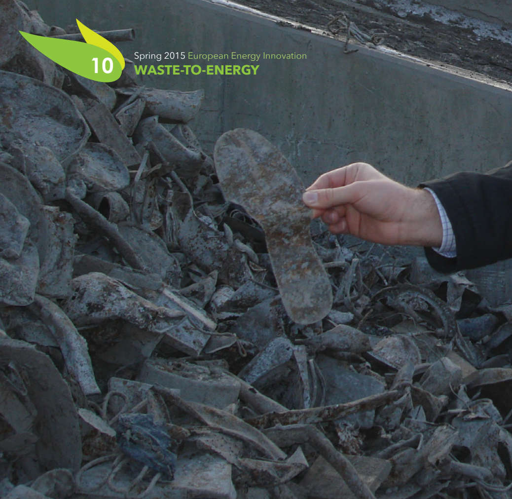
An example of recovered metals (in particular the metal sole of a safety boot)
