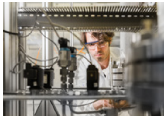
Assembly of Pressure Swing Adsorption System (rights by Photograph: www.eventfotograf.in / ©JRF e.V.)
