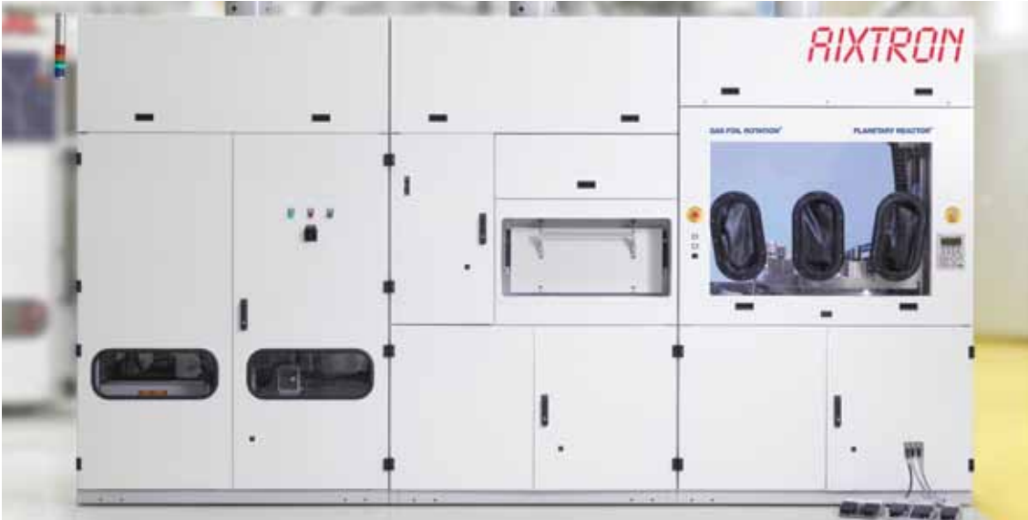
Europe has world leading positions all along the LED supply chain. Pictured is a reactor from Germany based AIXTRON, world leader of MOCVD equipment used for LED Manufacturing.
