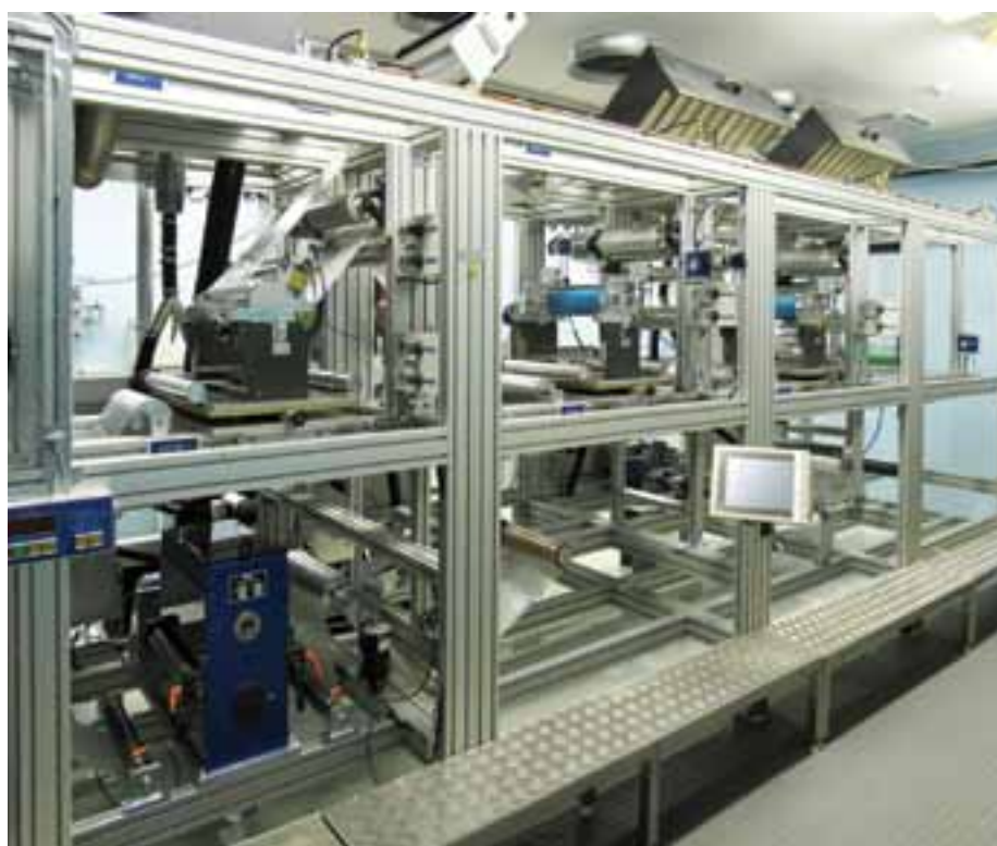
Figure 4. Modifiable ROKO R2R printing machine
