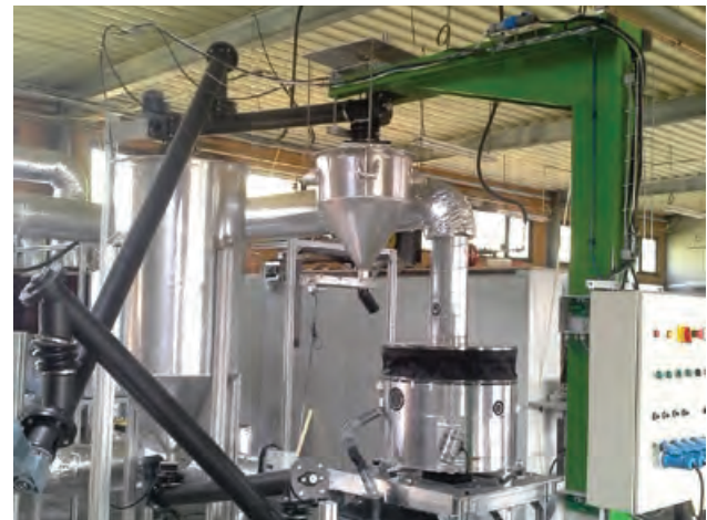
SOTHERCO test bench for seasonal heat storage technologies
