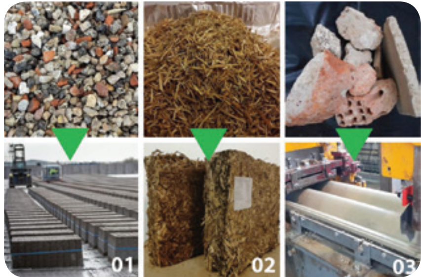
Examples of the RE 4 components: 01 – Concrete building blocks made of CDW mineral aggregate; 02 – Insulation panels made of CDW wood fibers; 03 – Reconstituted roof tiles made of CDW bricks and tiles
