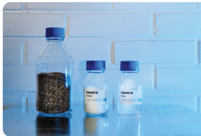
Figure 1. Collecting FT-wax from the synthesis unit MOBSU. Crushed bark, FT liquid product and FT wax.
