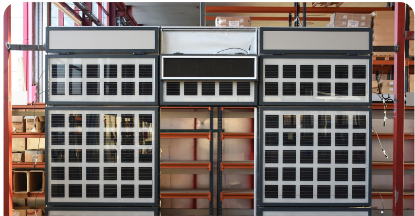
Figure 1. Integration of photovoltaic technology on synthetic stone in a full-scale prototype of the façade system. The horizontal registrable area interconnecting the three modules is displaced in the top part.
